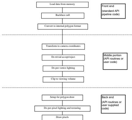
Figure 1: Standard Rendering Pipeline
